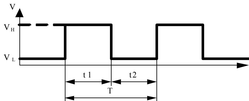
1. Period :  $T = \frac{1}{f_{\text{PWM}}} = t_1 + t_2 \text{ (sec)}$
