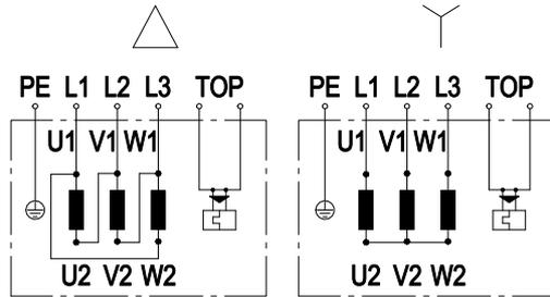
Note: Change of rotation direction by reversing two phases
