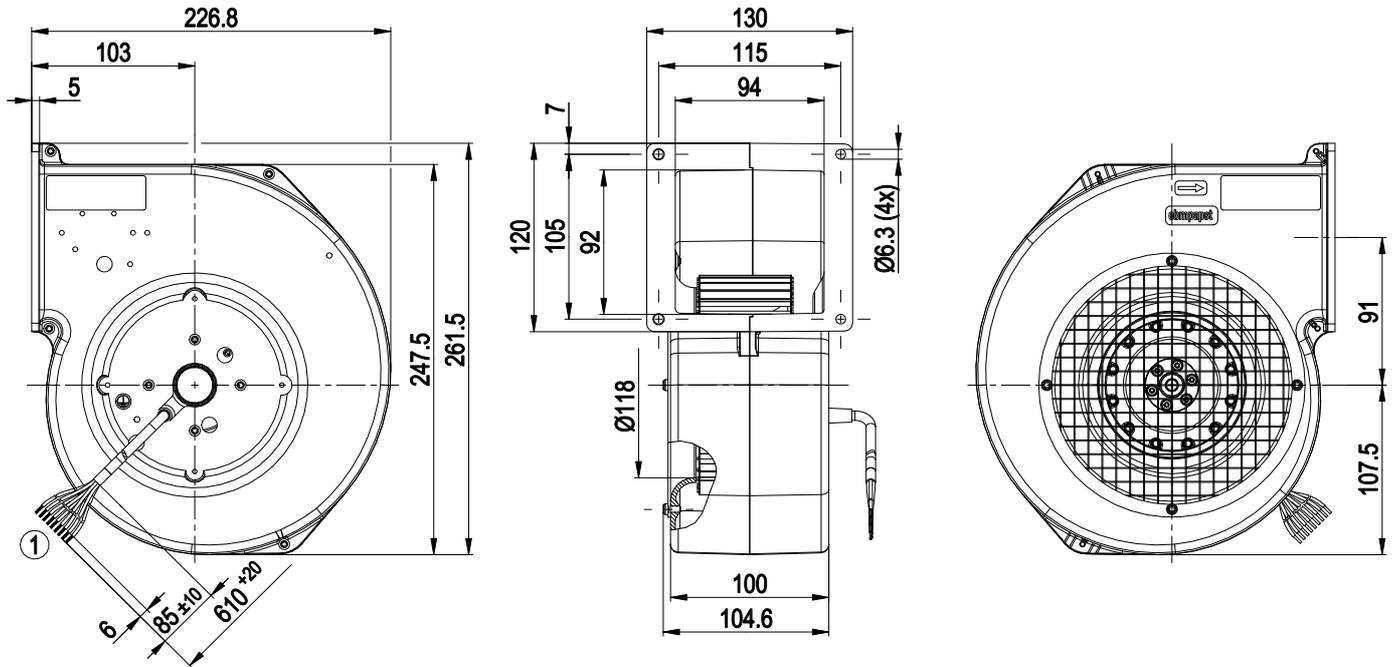
1 Cable silicone 9G 0.5 mm<sup>2</sup>, 9x crimped splices
