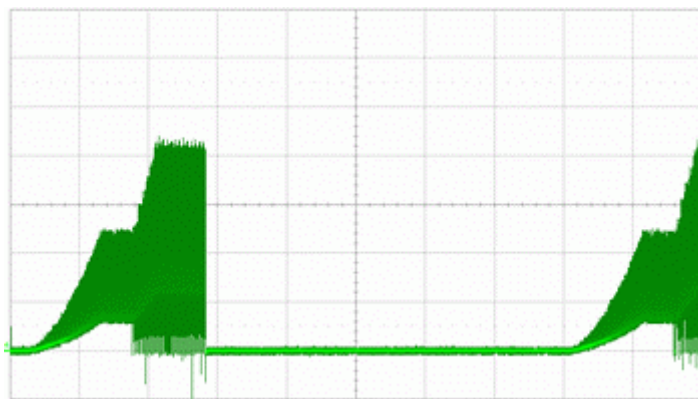
Locked rotor current @ 48 V ( I = 500\text{mA/div} ; t = 2\text{s/div} )
