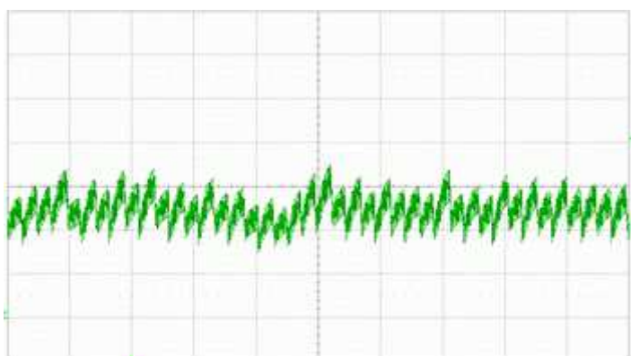
Running current at 48,0 V; 7.000 1/min; I=500mA/Div, t=2ms/Div
