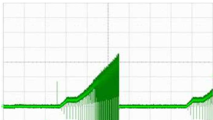
Locked rotor current @ 24 V (I = 1A/div ; t = 1s/div)
