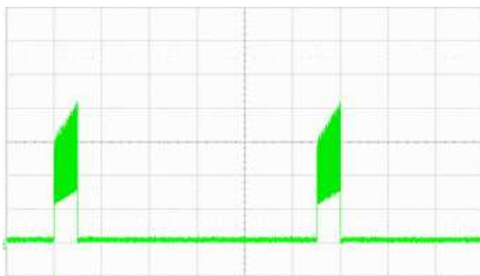
Locked rotor current @ 24 V ( I = 200\text{mA}/\text{div} ; t = 1\text{s}/\text{div} )
