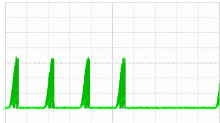
Locked rotor current @ 48 V ( I = 500\text{mA/div} ; t = 10\text{s/div} )
